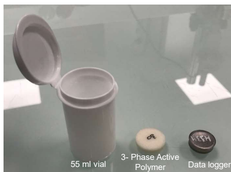
Figure 1. Experimental setup of container closure system for 3-Phase Active Polymer systems.
