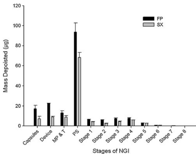
**Fig. 10** *In vitro* stage-by-stage deposition of FP and SX following aerosolization of combination DPI formulations containing micronized FP sample C from a Cyclohaler DPI device into a NGI at 90 L/min.
