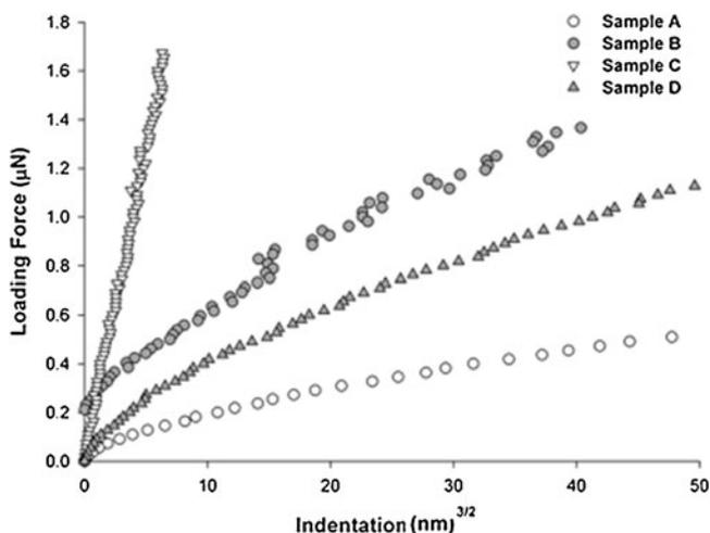
**Fig. 5** The measured loading force against indentation depth<sup>(3/2)</sup> for each sample of crystalline FP.
