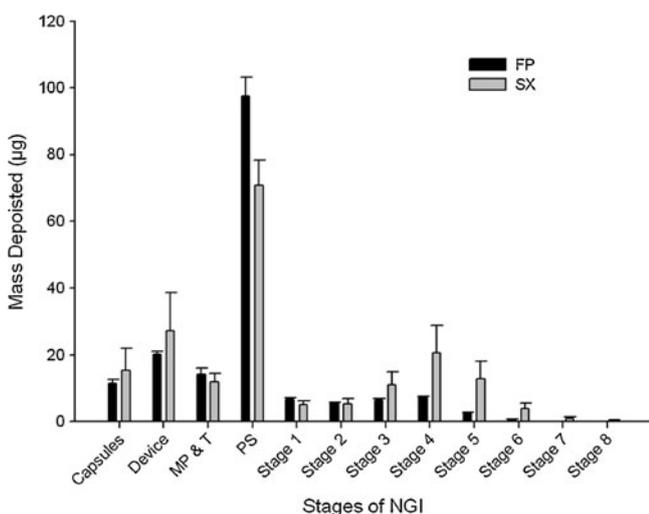
**Fig. 9** *In vitro* stage-by-stage deposition of FP and SX following aerosolization of combination DPI formulations containing micronized fluticasone propionate sample A from a Cyclohaler DPI device into a NGI at 90 L/min.
